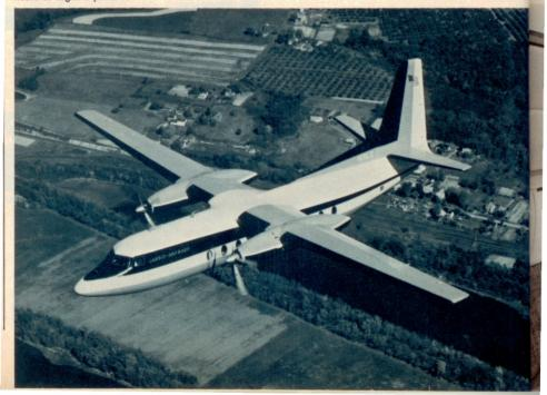
Gross weights are listed at 42,000 pounds for takeoff and 40,000 pounds for landing. The aircraft has a cruising range of 1,800 miles with a payload of 5,000 pounds at 14,200 r.p.m.
